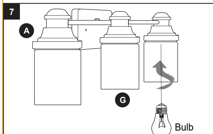
**Use 60-watt max. standard-base incandescent bulbs or CFL/LED equivalents.**
