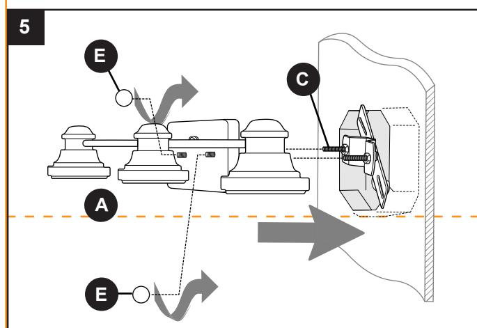
**E** Do not overtighten F as glass may crack or break.
