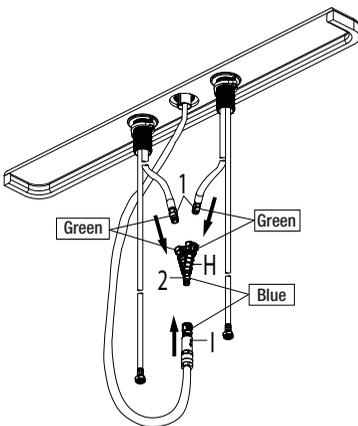
Connect the quick connector assembly (H) with the green tag to the receiving blocks (1) with a matching green tag. Push the quick connector (H) with the blue tag firmly upward and attach it to the receiving block (2) with a matching blue tag. Push firmly together until they snap into place.
