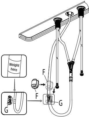
Install the weight clip (G) at the point of the hose marking "weight here". Insert the weight (F) onto the weight clip (G) by sliding it down onto the weight clip (G).
