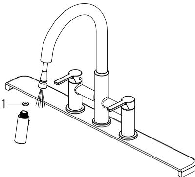
**Flushing and checking for leaks:** After the installation is complete, unscrew and remove the spray head in order to flush the line. Turn on the water supply and allow both hot and cold water to run for at least one minute each. This flushes away any debris that could cause damage to internal parts. Check for leaks. Reattach the spray head. Do not lose the washer (1) in the hose.
