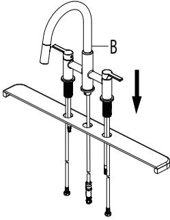
Shut off the water supply. Insert faucet body (B) through the hole in the sink.
