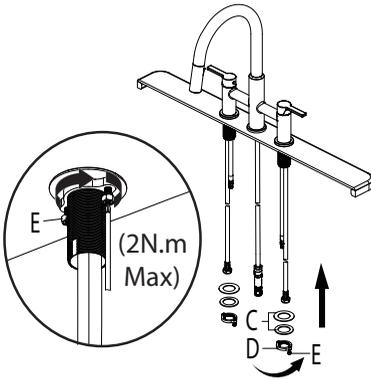
Install the washers (C) onto the threaded mounting shank. Thread the mounting nut (D) onto the mounting shank. Lock the mounting nut (D) into position by tightening the screws (E). Do not overtighten.
