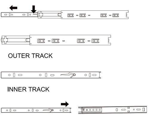
Align the outer track with the center of the inner track and push in.
