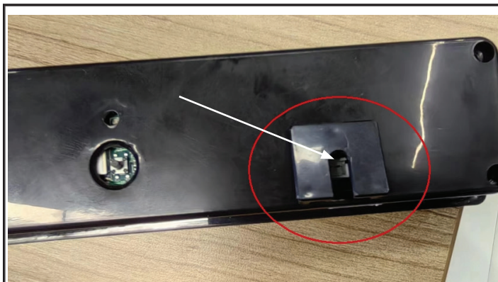
Figure 2 Install Display Panel Cord
