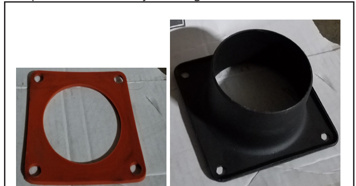
Figure 5: Exhaust Duct Adapter & Gasket
