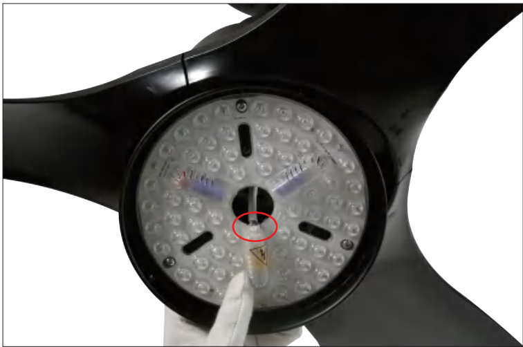
Step 14 Connect the wire to the Light source.
