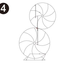
The rings at the junction of the first ball and the second ball are fixed with tie straps.
