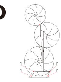
Two rings at the junction of the iron tube on the top of the third ball and the second ball are fixed with tie straps and four ground nails are inserted into the base.
