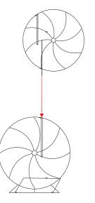
The latch at the bottom of the second ball is inserted into the iron tube at the top of the first ball.
