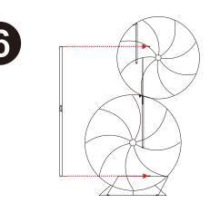
The support rod latch is inserted into the round tube between the first and second ball.
