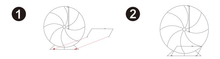
The base wire is inserted into the round tube of the frame.
