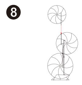
The wire latch at the bottom of the third ball is inserted into the iron tube at the top of the second ball.
