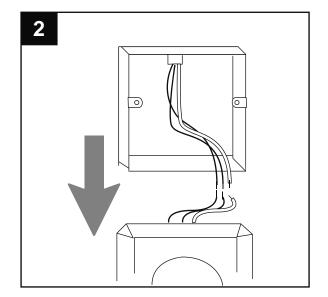
Remove mounting plate (B) from fixture (A) by removing mounting plate screws (D) from the edges of the fixture (A). Save mounting plate screws (D) for later use.
