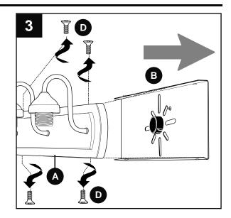
4a. To mount the item directly to an outlet box (not included), first attach mounting plate (B) to outlet box using the existing washers and outlet box screws or the machine screws (BB). Note: If the outlet box screws required for your outlet box are of a different size than the machine screws (BB), consult with a licensed electrician before proceeding.
