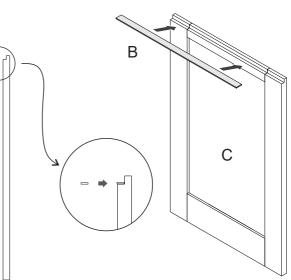
The Mounting Plate is to make sure there is a distance of 1/8" between the upper and lower door panels.
