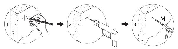
Install anti-tipping device as shown.
