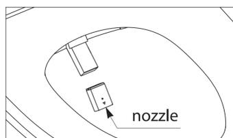
Powered on and not seated: Press the "Nozzle Clean" button on the remote controller, and the washer will automatically extend. If there is dirt in the nozzle orifice, you can gently hold the washer with one hand and clean it with a toothbrush with the other hand.
