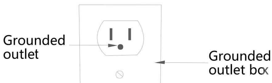
**\*WARNING: Risk of electric shock Connect only to a circuit that is protected by a ground-fault circuit-interrupter (GFCI).**
