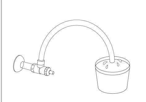
Open the angle valve for water supply. The measured water flow for 10 seconds should exceed 3L.
