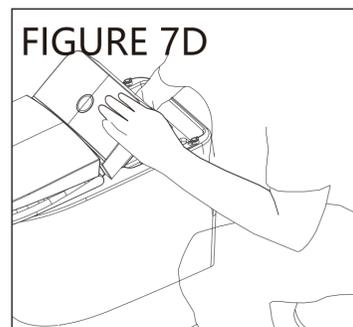
**Caution:** Do not move the toilet bowl around once the toilet bowl is in position. It can damage the wax ring seal and result in water leakage.
