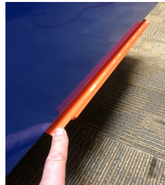
Mounting bracket installed loosely on roller cabinet.
