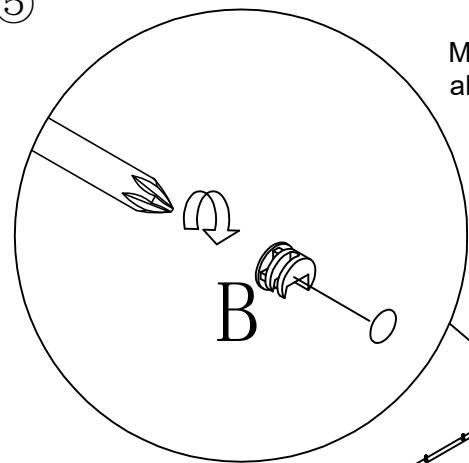
Make sure the arrow on the screw align to the hole on the side.
