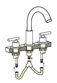
4. Push the blue button on the quick connect hose and insert the hose to the faucet and the handles' pipe as photo 4
