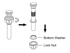
1. Unscrew the lock nut and bottom washer from drain stopper
