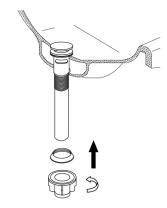
3. Re-screw the bottom washer and lock nut onto drain stopper
