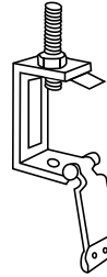
A853 Channel Hanger Use hanger rod 3/8" or 1/2". Use with "A", "B" or "C" series single channel.
