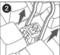
Use the key switch puller tool to push in the two tabs located on both sides of the switch. Once pushed in, pull upwards to remove the switch from the board.
