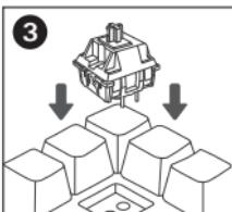
Select a switch and examine the copper pins at the bottom of the switch to ensure they are straight. Align the copper pins with the sockets on the pad. Insert by pushing straight down.
