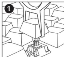
Use the keycap puller tool to clamp a keycap and pull upwards to remove.
