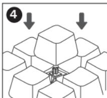
Align the keycap with the switch stem and press down gently to insert.
