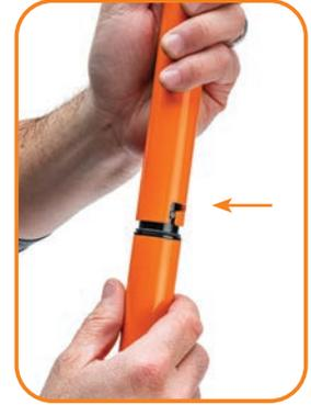
Turn the lower tool body clockwise to lock it into place.
