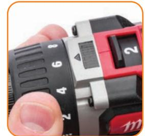
If your drill has a drill and clutch mode, set it to clutch mode. Turn down torque to the lowest setting. Increase as necessary.
