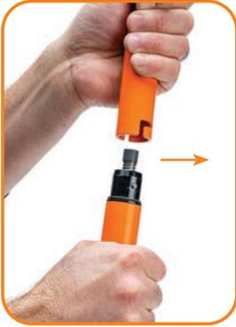
Separate the tool by turning the lower tool body counter-clockwise and sliding the locking pins out of the notches.
