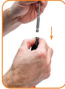
Pull back the collar, then insert the T-15 bit and release the collar to lock the bit in place.
