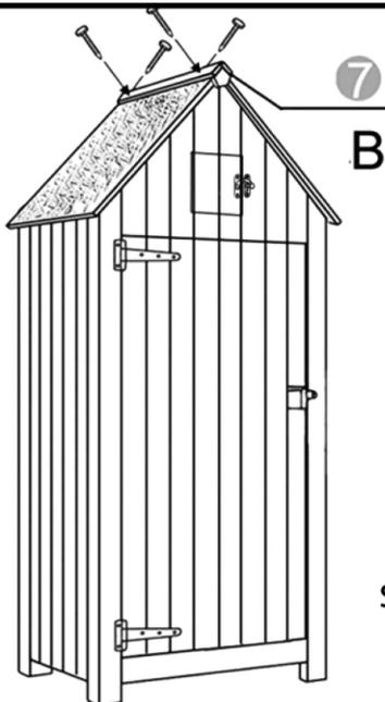
Secure roof cap part ⑦ by using 4x screw (B).
