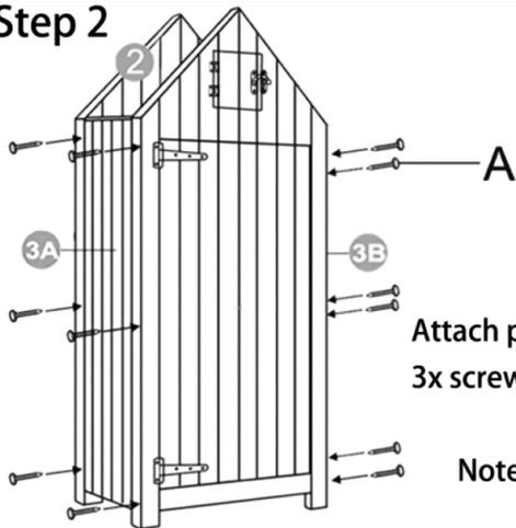
Attach part ③A to part ① finished in step 1, secure with 3x screw (A); Attach part ② to ③A, using 3x screw (A). Repeat for the right side panel part ③B using 6x screw (A).
