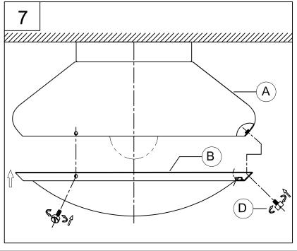
7. Attach the glass shade assembly (B) to the fixture (A) using the three slotted finial knobs (D) and secure modestly tight.
