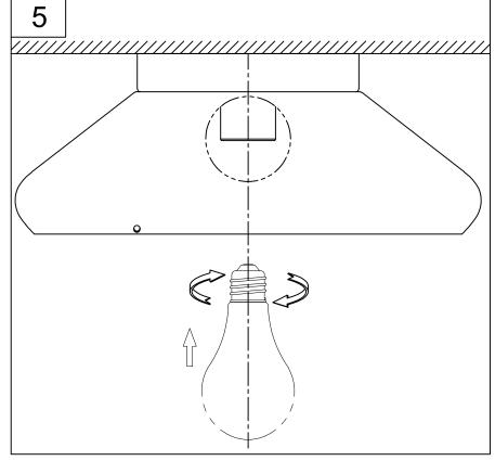
5. Thread the lamp (not included) into the fixture socket. Use 60-watt MAX incandescent medium base lamp, or equivalent SBCFL or SBLED.
