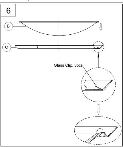
6. Attach the glass shade (B) to the metal ring (C), bend the three glass clips over onto the glass edge to secure tightly.
