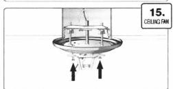
16. Lift the fan and capture its ball joint in the fan hanger bracket. Cut off any excess wiring.
