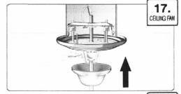
Raise the fan canopy to the fan hanger bracket Secure the canopy in place by using the two canopy's attachment screws.
