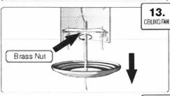
14. Screw the mounting plate onto the threaded pipe so that the plate rests against the heads of the screws on the mounting bracket. Thread the second nut through the wires. Screw the brass nut up the threaded pipe all the way to the mounting plate. Tighten the brass nut to secure the mounting plate to the threaded pipe.
