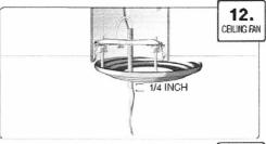
Remove the medallion. Screw the brass nut onto the threaded pipe all the way up to the mounting bracket and tighten the brass nut.
