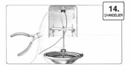
15. Using wire nuts, pair together the fixture's hot wire to the power-outlet-adapter's hot wire, the fixture's neutral wire to the power-outletadapter's neutral wire and the fixture's ground wire to the ground wire on the mounting bracket. Tuck the wiring neatly into the light canopy and medallion
