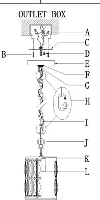
Step A1: By measuring, determine the correct number of links needed for proper hanging height. Using the chain pliers, disconnect and discard the unwanted part.
