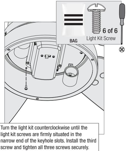
Turn the light kit counterclockwise until the light kit screws are firmly situated in the narrow end of the keyhole slots. Install the third screw and tighten all three screws securely.
