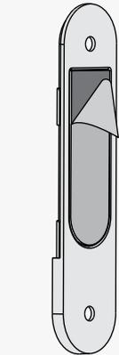
Separate the lining from the back of the adhesive strip on the cradle bracket.
