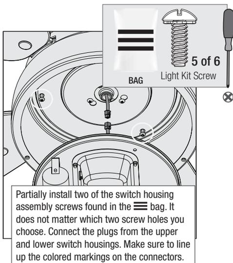
Partially install two of the switch housing assembly screws found in the hardware bag. It does not matter which two screw holes you choose. Connect the plugs from the upper and lower switch housings. Make sure to line up the colored markings on the connectors.
