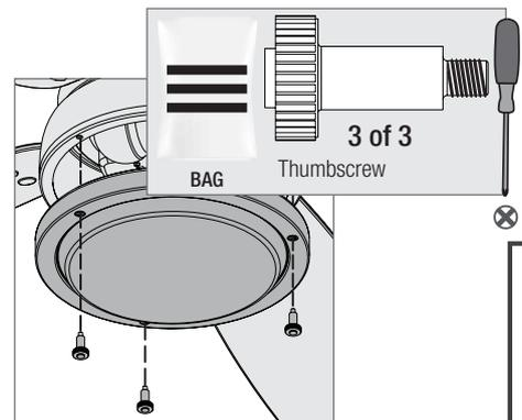
Lift the globe assembly and attach it to the upper switch housing using the three thumbscrews, found in the hardware bag. Tighten all three screws securely by hand.
