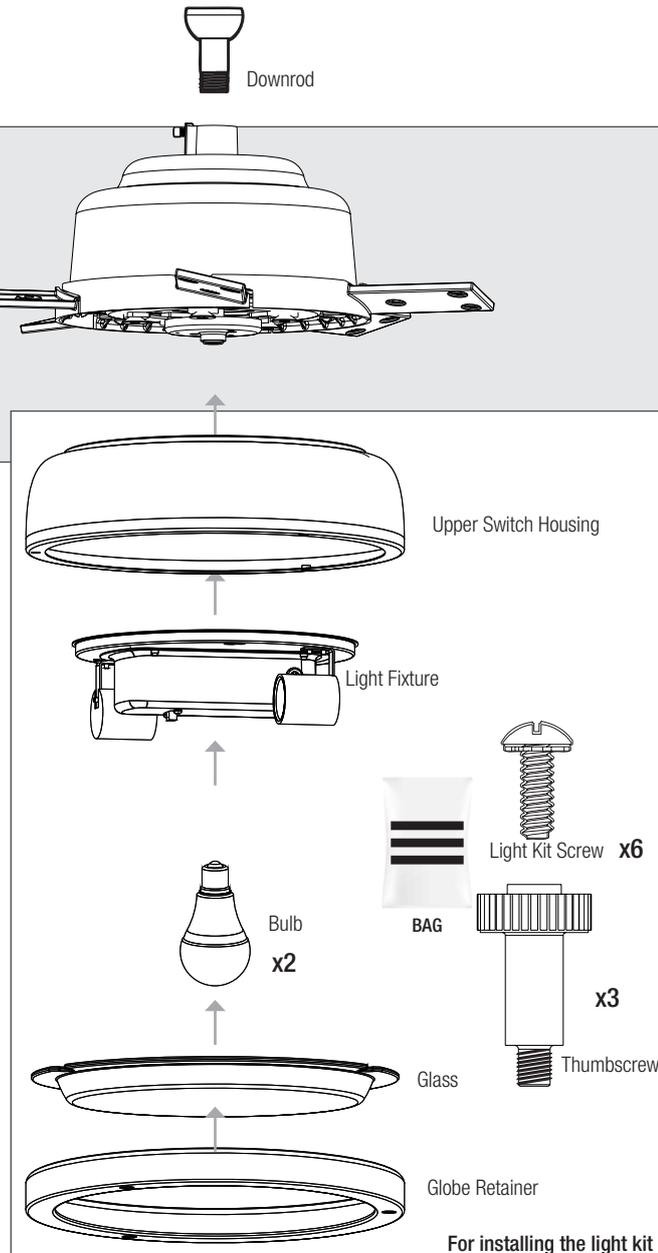
For installing the light kit
