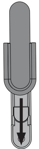
Slide the cradle onto the mounted bracket.
