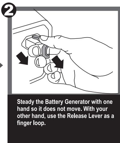
Steady the Battery Generator with one hand so it does not move. With your other hand, use the Release Lever as a finger loop.
