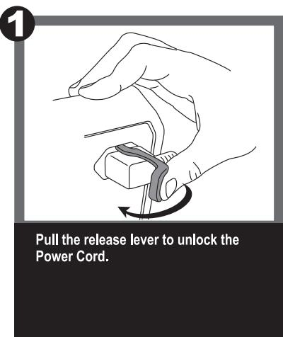
Pull the release lever to unlock the Power Cord.
