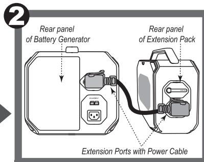
Connect your Power Cable to the Battery Generator and the Extension Pack. Both units will now begin charging together.
