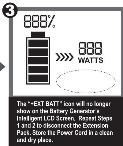
The "+EXT BATT" icon will no longer show on the Battery Generator's Intelligent LCD Screen. Repeat Steps 1 and 2 to disconnect the Extension Pack. Store the Power Cord in a clean and dry place.
