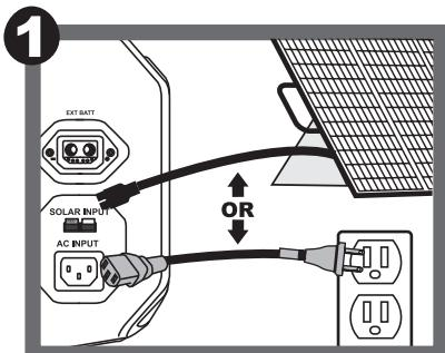
Plug the Battery Generator into AC and / or solar power.
