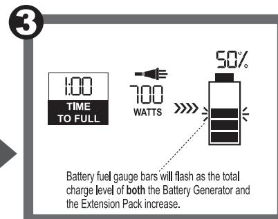
The fuel gauge will flash as both units charge. The fuel gauge now displays the combined battery level of both units.
