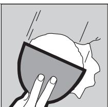
Apply a skim coat of joint compound with a joint finishing knife to damaged area and feather to get a smooth finish. Let dry and apply second coat if necessary.
