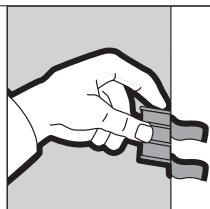
Slip drywall repair clips onto the edge of the wallboard opening.
