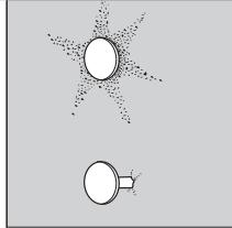
To repair a popped fastener, drive and dimple 1-1/2 in. from popped fastener. Remove popped fastener. Cover with joint compound. Sand and prime when dry.
