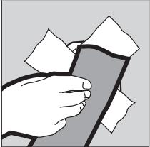
Crisscross two or three strips of joint tape over opening and embed tape in joint compound. Let harden.
