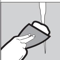
Trim any loose material and wipe clean. Apply compound to crack with 6 in. finishing knife.
