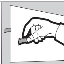
Remove tabs from each drywall repair clip. Apply compound and tape to all four section sides. Do not overlap tape. Apply second and third coats of joint compound, allowing each coat to dry before applying next coat and feathering out from previous coats. Sand and prime when dry.
