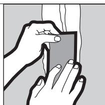
Embed tape in compound to bridge crack. Draw knife firmly over crack to tightly embed tape. Let compound harden.
