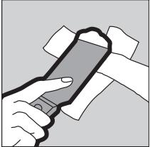
Apply coat of joint compound over taped area. Let harden and apply second coat. Sand and prime when dry.
