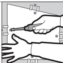
Insert new drywall section into area removed from existing wall. Position fasteners about 3/4 in. in front of the edge and centered between the tabs. This will line up the fasteners with perforations in the clips. Screw through new drywall into each drywall repair clip.
