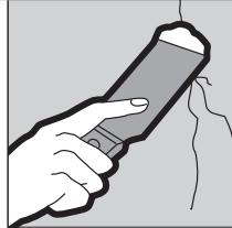
To repair a small hole or crack, wipe area clean. Fill with joint compound, using a putty knife. Let harden. Add second coat if necessary. Sand and prime when dry.
