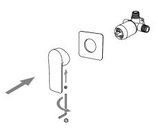
6.(1) Twist some Teflon tape on the adapter and screw it to the water pipe with big Allen key. Inset spout to the adapter then tighten it with screws.
