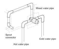
4.Switch on/off the cartridge, check all connectors without any leakage. And then seal the wall and take off protection cover.
