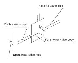
Recommended depth for installing shower valve body before tiling tiles: 40-50mm. Note: Tile opening should be bigger than shower valve diameter at least 5 mm.
