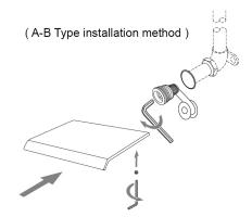
6.(2) Twist some Teflon tape on the adapter and screw it to the water pipe with big Allen key. Install the two fixed joints on both sides of the adapter as picture shows. Inset spout to the adapter then tighten it with screws.
