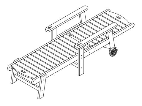
The backrest has five adjustable levels. Rotate the latch to loosen backrest adjuster, then adjust the gear position to the angle which you want.
