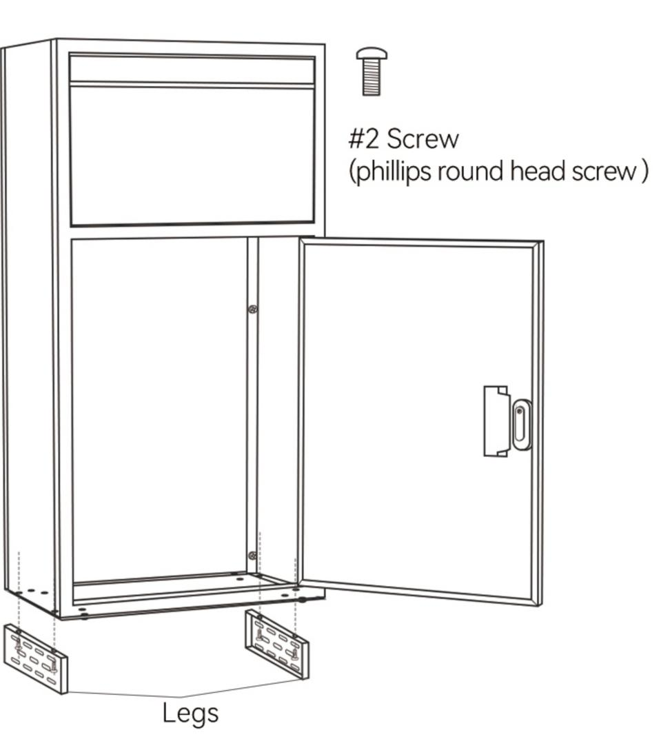
Attach the two legs to the left and right sides of the bottom panel. Tighten the connection holes using #2 screws.
