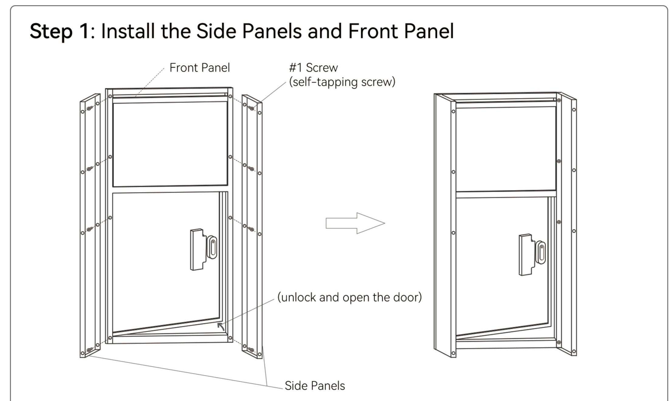
Align the two side panels with the front panel, matching the holes, and tighten with #1 screws. (When installing the side panel near the door lock, unlock and open the door first to allow the screws to align with the corresponding holes.
