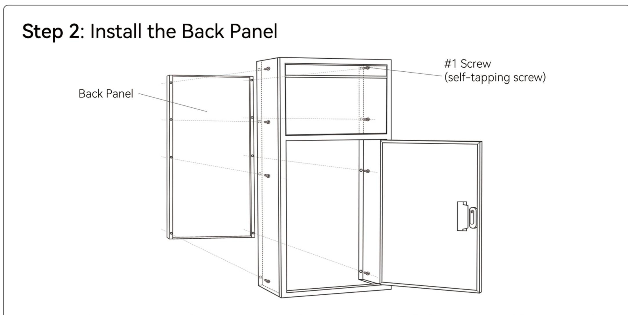
Align the back panel with the two side panels and tighten with #1 screws.(It is recommended to open the front door for easier access to the screw holes.)
