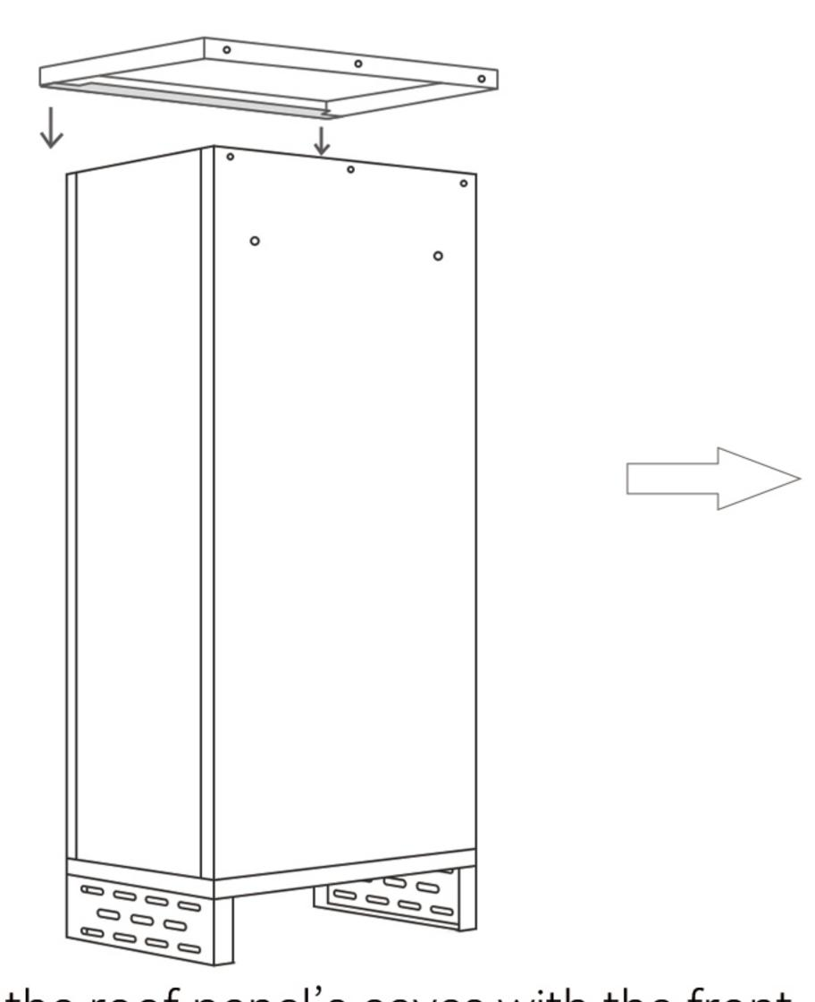
Align the roof panel's eaves with the front of the delivery box, then press firmly from the front to the back to ensure the roof panel fits onto the box's main body.
