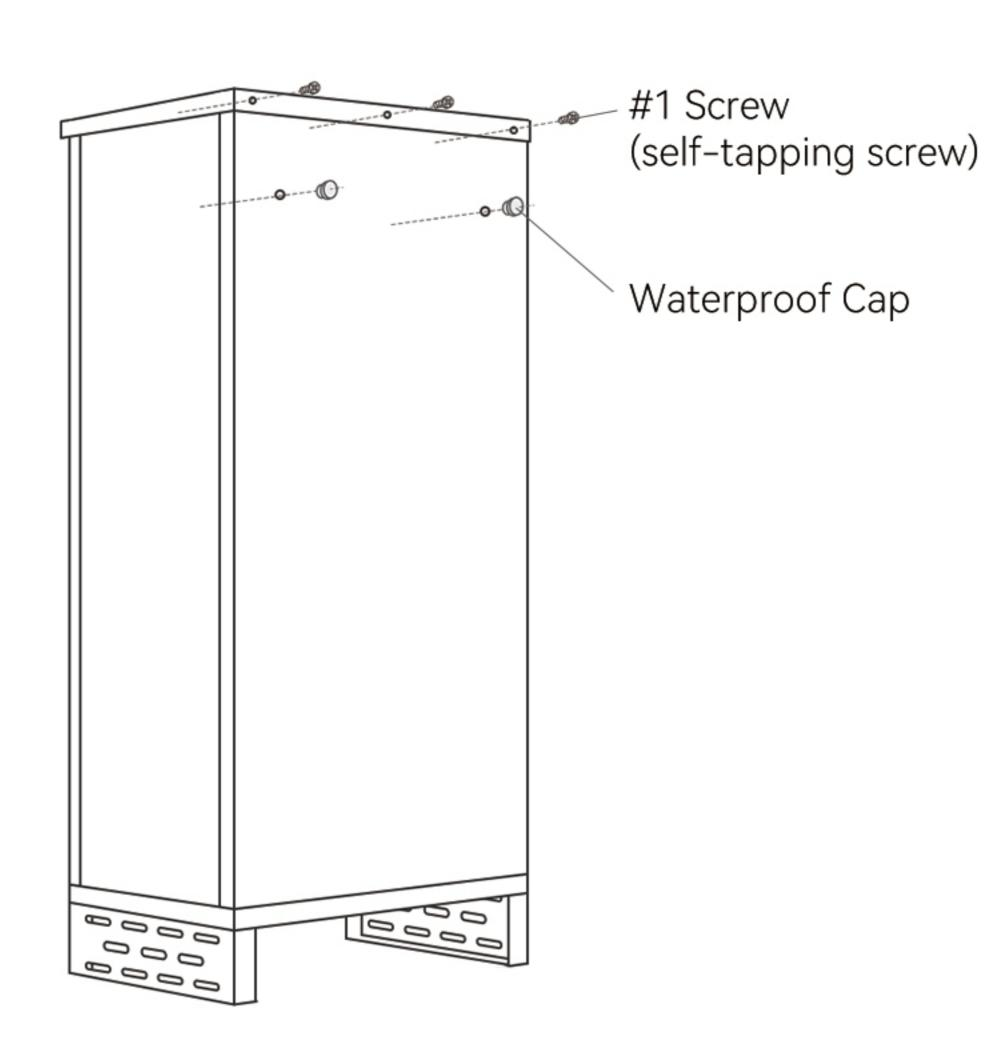
Secure the screws at the back of the roof panel and attach the waterproof cap.
