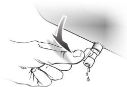
Drain valve (open)
