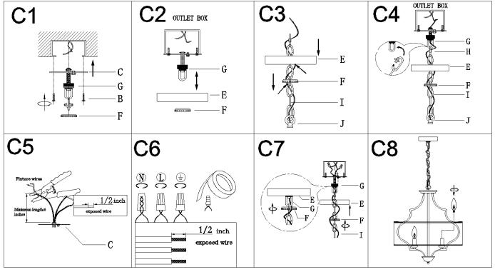
Step C1: Remove collar ring (F) from collar loop (G). Attach single bar (C) to the outlet box with mounting screws (B). Note: the side of single bar marked "GND" must face out.
