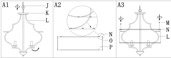
Step A1: Screw loop (J) onto the top of cover (K).
