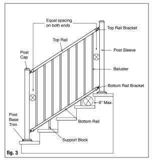
**Step 7** Mark location of the bracket base screw holes on the post. Include the bracket side cover when determining the center location. Predrill through the post, using a 9/64" drill bit. Position the base of each bracket with the bracket cover side facing the stairs, and attach to the post with two screws.
