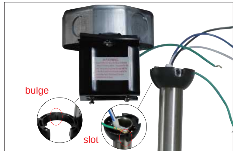
Step 11 Hang the fan on the hanging bracket and align the slot on the downrod with the bulge on the hanging bracket.
