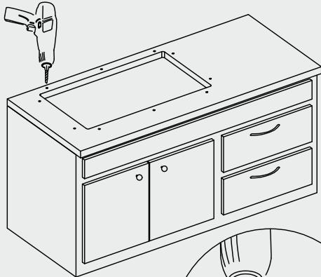
Drill 3/8" diameter x 1/2" deep hole in the countertop. Loosely install the fasteners.
