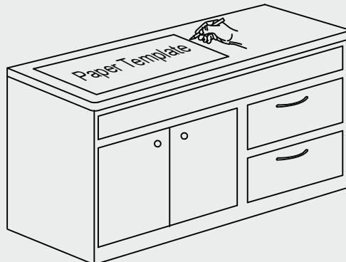
Place the template on the counter, in the location where you will be installing the sink. When placing the template, note the location of cabinet doors and panels to ensure that they are compatible with sink installation. Make sure that there is enough space for water supply installation. Identify the location of the faucet and soap dispenser. Fix the template to the counter using masking tape. Trace the template with a marker pen.
