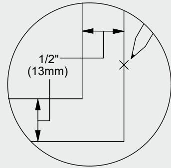
Turn countertop over and align the sink with the countertop. Decide the locations for mounting brackets. Mounting holes should be 1/2" from the edge of the sink.
