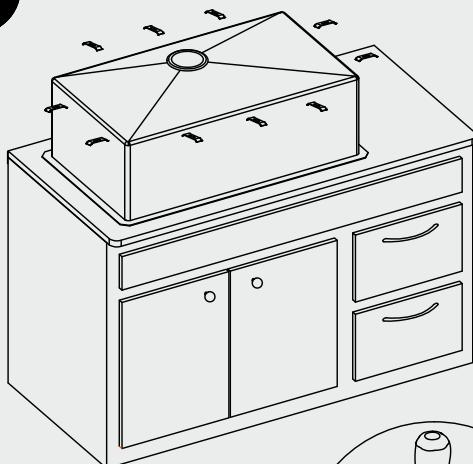
Attach mounting hardware to secure bowl. Remove excess sealant from inside lip. Allow sealant to set for 30 - 60 minutes.
