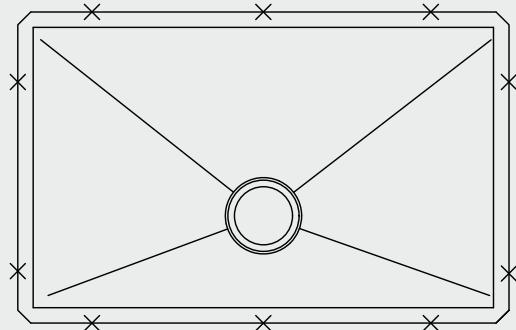
Cut the opening in the countertop by carefully following the traced line. Cut the countertop using the appropriate cutting tools.
