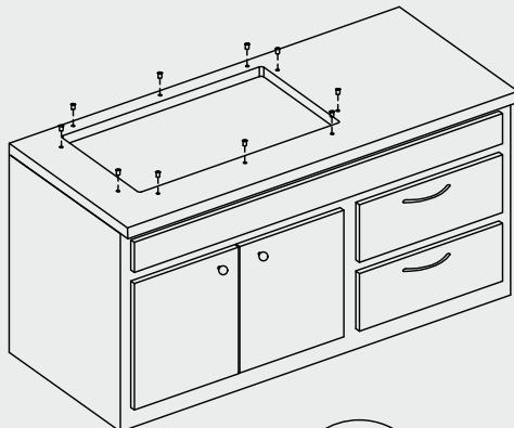
Insert anchors into the drilled holes and lightly tap with a hammer until flush.
