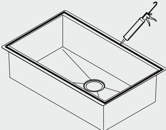
Apply a quality silicone to the underside of the countertop around the perimeter of the sink rim. Position and align the sink in the correct position over the opening and press firmly.
