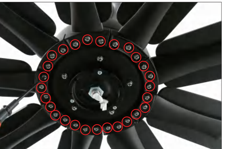
Step 17 Install the Blades to the motor.
