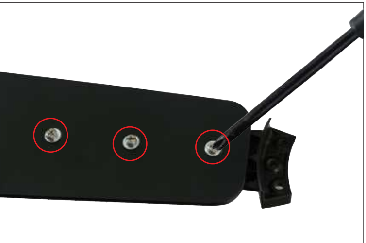
Step 16 Install the Blade to the Blade Holder.
