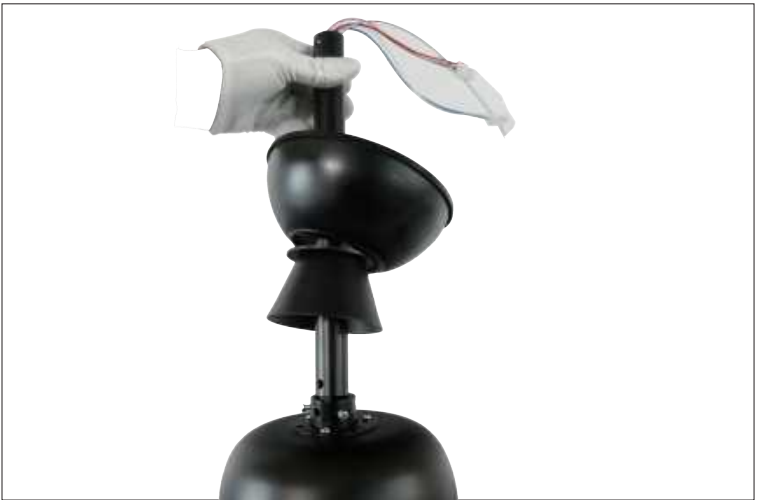
Step 7 Install the up canopy, canopy cover and down canopy to the downrod. Feed the wires from the motor to downrod.
