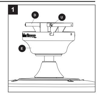
Secure the canopy (E) with the mounting bracket screws (U) previously removed (Step 4, page 8).
