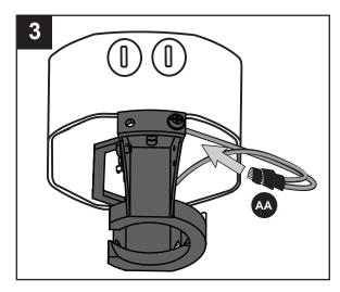
Align the canopy (E) over the loosened mounting bracket screws (U) preassembled on mounting bracket (D). Place the keyholes of the canopy (E) onto the mounting bracket screws (U) and rotate the canopy (E) clockwise.
