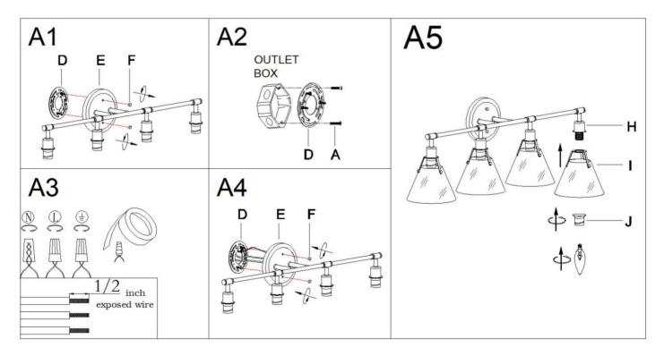
Step A1: Unscrew knob nuts (F) from back plate (E), then set them aside for later installation. Step A2: Carefully pass the supply wires from the outlet box through mounting plate (D). Secure mounting plate (D) to the outlet box with mounting screws (A).
