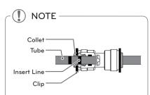
Gently press the Collet and insert the tube until only one line shows on the tube.
