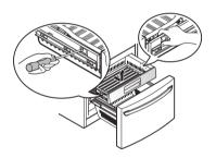
3 Remove the screws from the rails at both ends.
