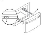
4 Insert the drawer into the frame, and push the drawer back into place until you hear a click.
