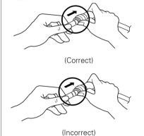
Pull the tube to make sure that the tube is tightly fastened and then insert the clip.
