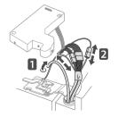
4 Rotate the hinge lever counterclockwise
