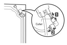
6 Make sure that the door-switch located inside the cover is tightly connected. Place the cover 1 in its position and tighten the cover screw 2.
