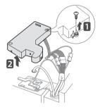
3 Remove the cover and pull out the tube **1**. Disconnect all wire harnesses **2**.
