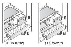
To install, slightly tilt up the front, insert the drawer into the frame and push it back into place.
