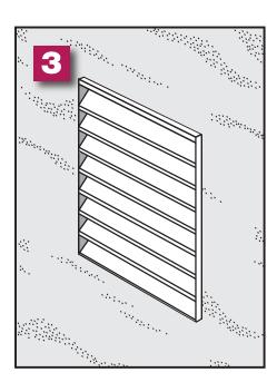
3) Finish with lath and plaster or siding material.
