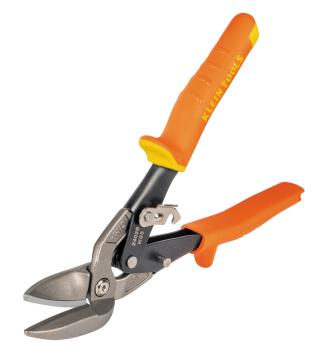
Cut and trim sheet metal in comfort with the Klein Tools straight cutting Offset Snips. Snip blades are made of forged, heat-treated steel for strength and durability. Offset blades make it easier to cut in tight curves and keep the user's hand away from the metal. The contoured plastic handles with thumb guards are color-coded by cutting pattern.
