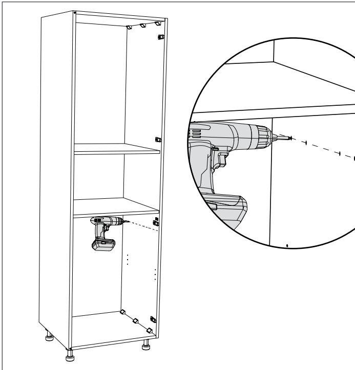
**5** Insert the slide and align the holes with the drilled holes on the cabinet. Using a power drill or screw driver fasten the side mounting slide to the cabinet using four M5x16mm Screws.
