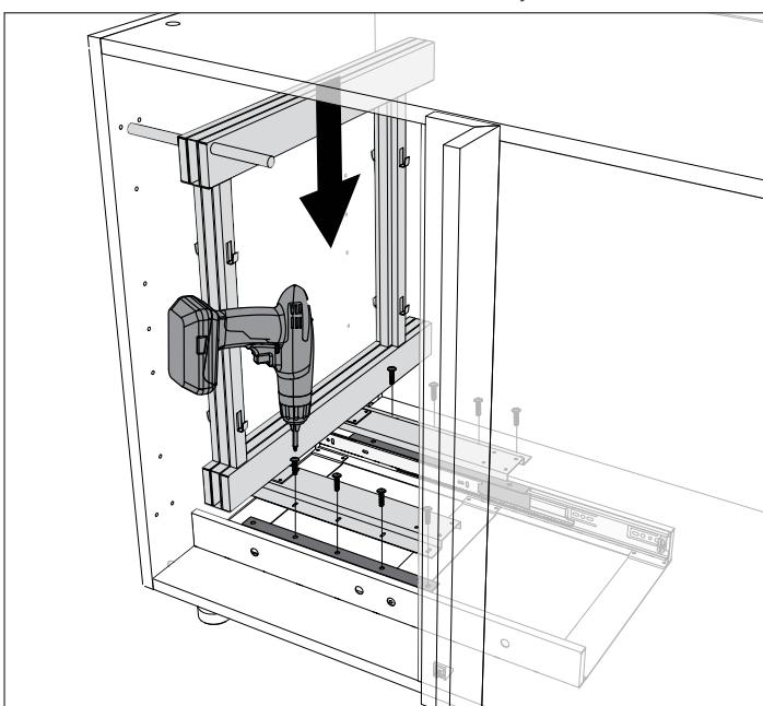
5 Slide the top frame and attach the handles using two M4x8mm screws. Attach bottom brackets (B) to the top frame using eight M5x8 screws included with the assembly and screw in the two handles on top.
