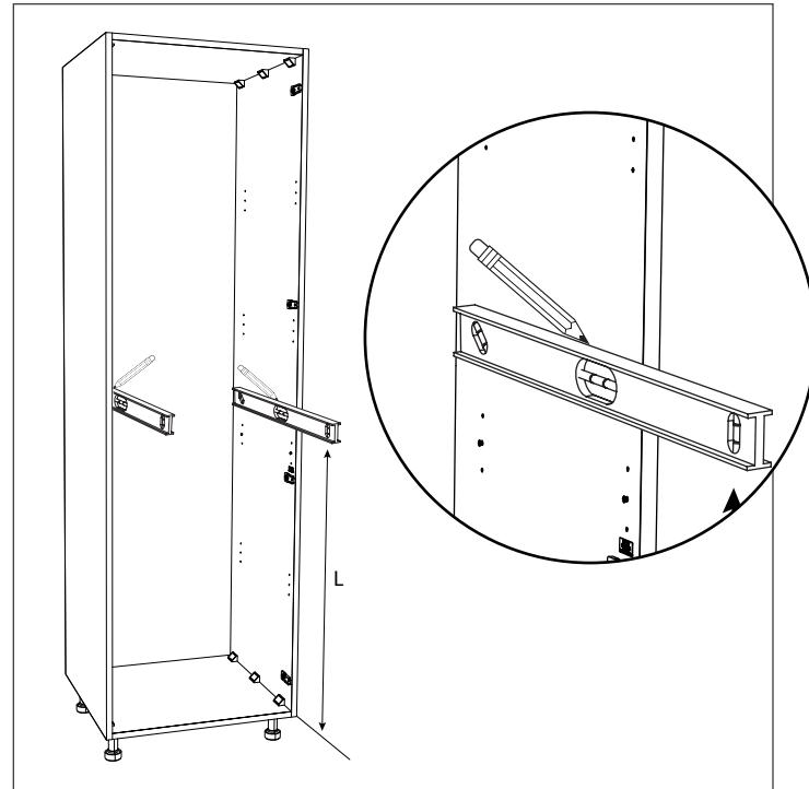
2 Mark a hole at 1.5 in from the front on the horizontal line.
