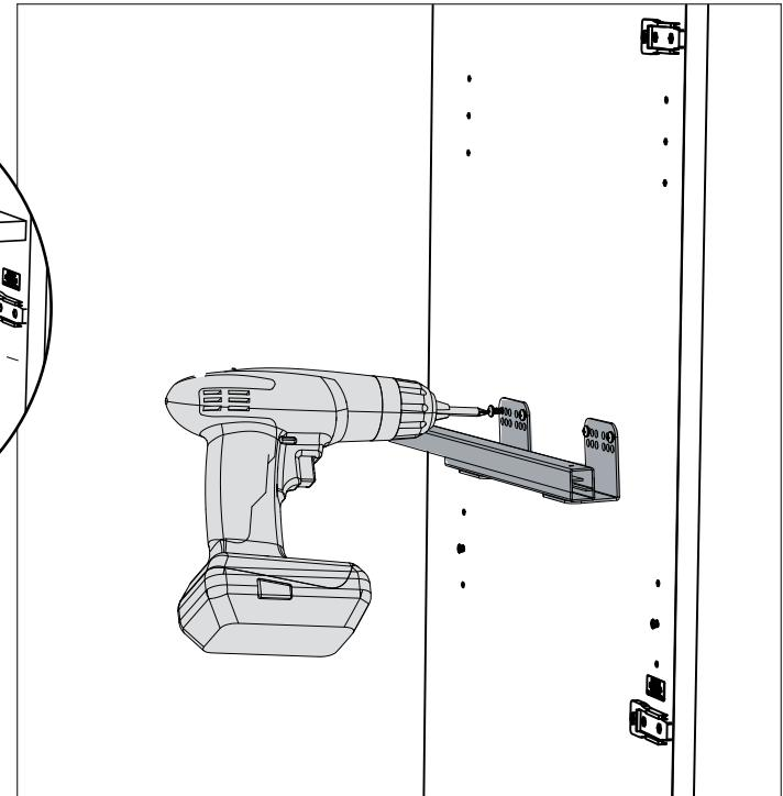
**6** Take the support frame and adjust the frame length by adjusting the screws at the bottom according to the interior of the cabinet. Make sure to adjust the distance of the four sides of the frame consistent.
