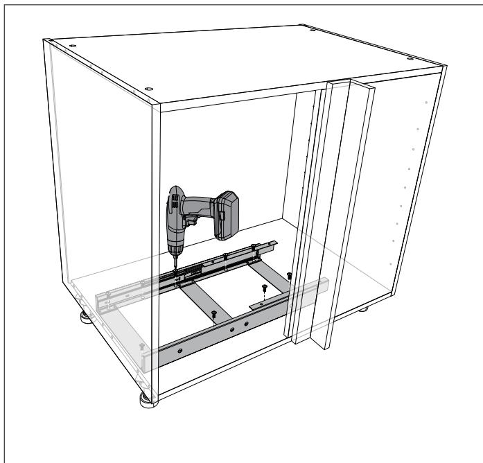
6 Insert the top frame assembly and align the bracket holes with the holes on the sliding base. Using a screwdriver or cordless drill fasten the top frame assembly using the eight M5x8 screws included with the assembly.
