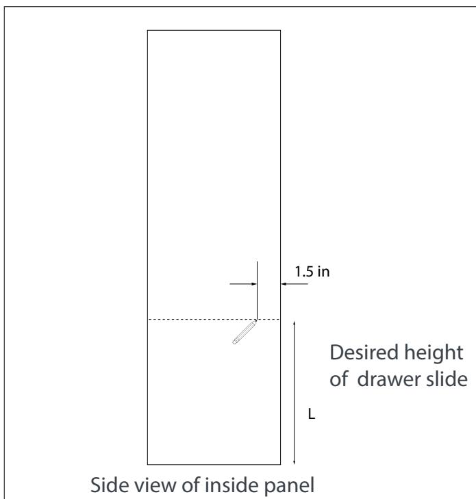
**3** Insert the side mounted slide and align the first hole on the slide with the marked hole position. Use the slide as template mark the outer holes of the slide mounting bracket.
