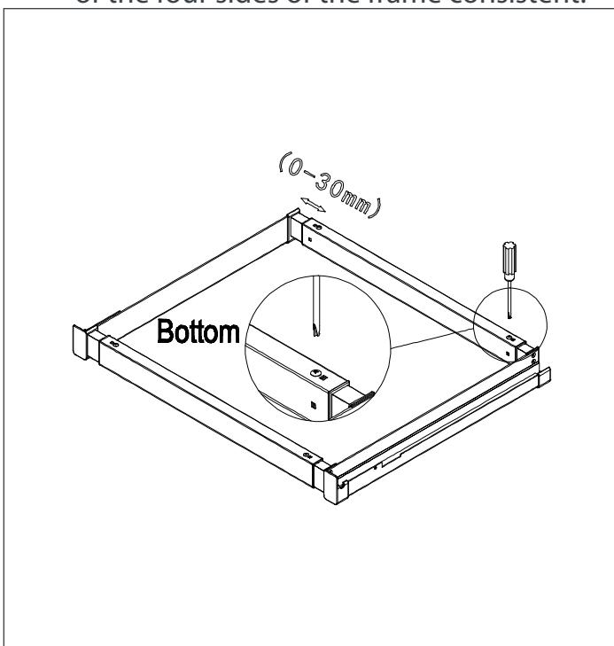
**7** Install frame on the slides. After the frame is installed, test whether the frame is sliding smoothly. Lock the four screws at the bottom of the frame.
