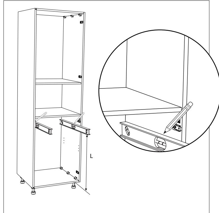
**2** Mark a hole at 1.5 in from the front on the horizontal line.
