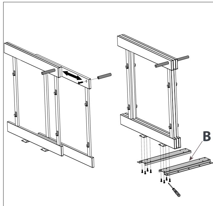
7 Slide the top frame assembly out and install the metal baskets.
