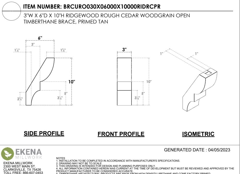
5. TIMBERTHANE ARCHITECTURAL PRODUCTS ARE MADE FROM HIGH DENSITY URETHANE AND COME FACTORY PRIMED WWW.EKENAMILLWORK.COM
