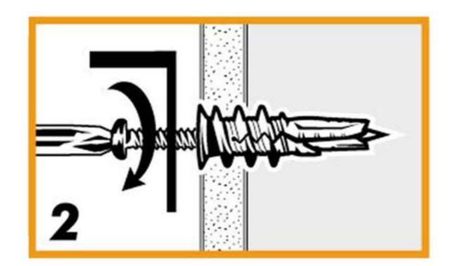
Insert screw through item to be hung and turn into anchor.
