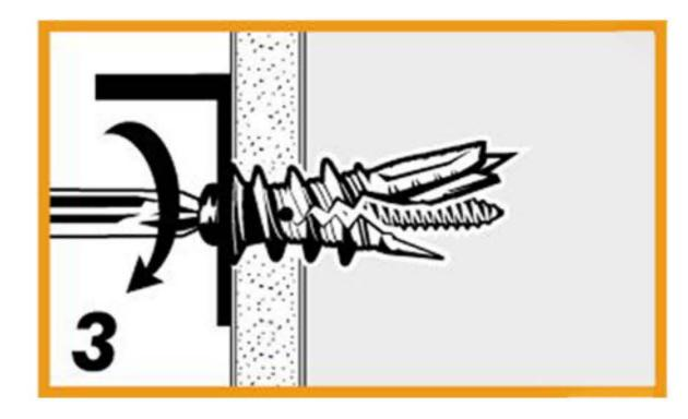
Anchor will "click" once when the screw is halfway in to indicate that the anchor is secure. Continue tightening until flush.
