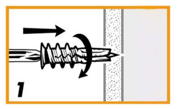
Using #2 Phillips screwdriver, press anchor tip slightly into drywall. Applying pressure, turn anchor until flush with drywall. Do not overtighten.
