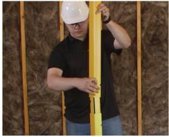
**5**. Fit the second boom section over the split boom connector. Align the corners access holes with those of the lower section.
