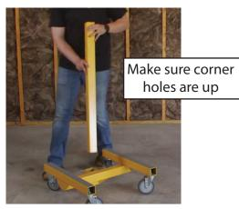
**1**. Install either of the boom sections into the dolly base. Make sure the holes in the corner of the tube are up.
