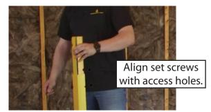
**4.** Insert the split boom connector. Align the set screws with the access holes in the boom tube.
