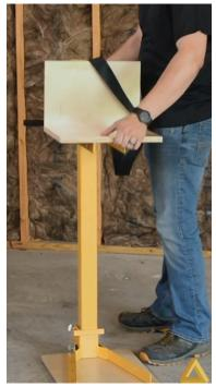
**3.** Let out a 2' loop of strap on the Collar Assembly and slide the Collar Assembly over the Boom Tube.
