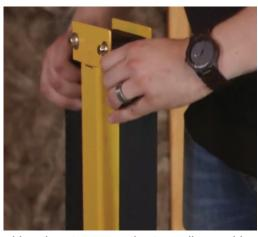
**5**. Position the strap over the top roller, making sure that it is aligned straight with no twists.
