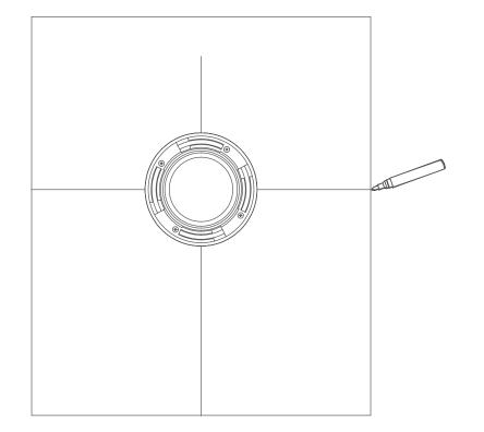
(3) Install smart toilet bottom flange anchor screw.
