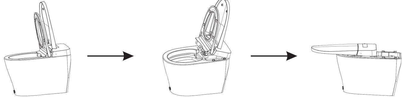
(6) Installing the toilet bowl onto floor flange
