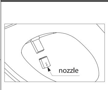
Powered on and not seated: Press the "Nozzle Clean" button on the remote controller, and the washer will automatically extend. If there is dirt in the nozzle orifice, If there is dirt in the nozzle orifice, you can gently hold the washer with one hand and clean it with a toothbrush with the other hand.
