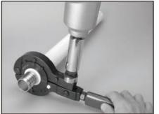
Drive the nut down with an impact wrench until blue LED light turns on.
