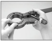
1. Open clamp, then press down on the keyed slot to loosen jaw.
