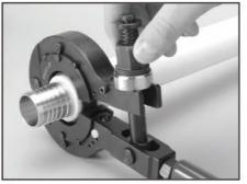
2. Load fitting assembly into the tool. Position tool so crimp ring is completely covered by tool jaws. Confirm tubing is at a 90° angle to the fitting and close jaw. Hand tighten the nut to hold fitting in place.
