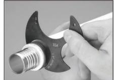
Check crimp using the supplied "Go Gauge".
