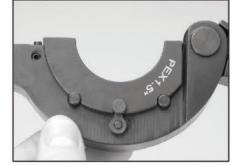
**4.** Rotate key back into position until key clicks to lock jaw in place. Repeat for other jaw.
