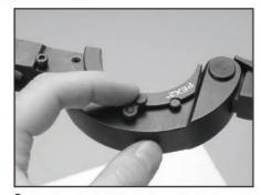
Continue to hold in the keyed slot, turn tool around and move key out of position. Remove jaw from clamp.
