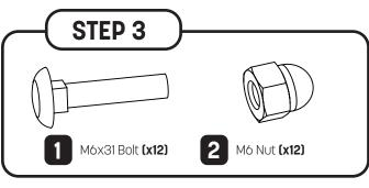
Secure each **cross bar** to the **frame legs** with 12 M6x31mm bolts **(1)** and 12 M6 nuts **(2)**.
