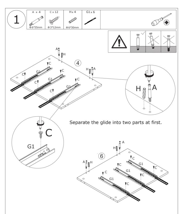
Fix slide rail(G1) into No.4 and No.6 plate respectively with screw(C) as shown.
