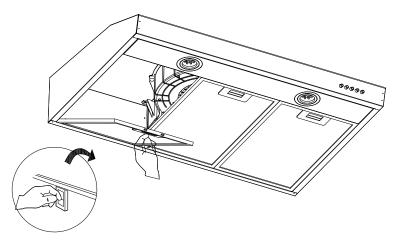
2. Plug the activated carbon filter into the blower as shown and turn it in anti-clock wise direction.
