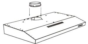
4) Align the air ventilation port of the range hood with the cabinet ventilation hole at the bottom, pass the power cord through the power hole, and then use four 0.16"\*1.18" screws to lock into the corresponding position of the pencil marked in the cabinet to fix the range hood.
