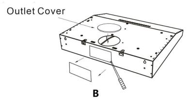
Install the air outlet assembly on the circular air outlet at the back of the range hood;
