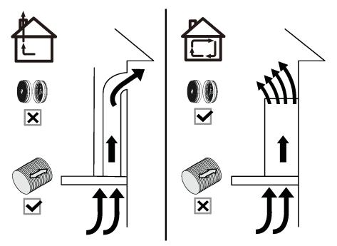
b) When possible, use at least 2 foot straight runs before any turns. Larger duct work may be required for best performance with longer duct runs.
