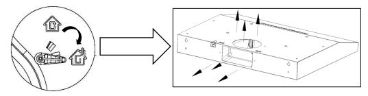
• Recycling: the recycling mode with activated carbon filter, Turn the adjuster to indoor position, install the outlet cover, turn on the range hood, then the air can be vented from the inside outlet.
