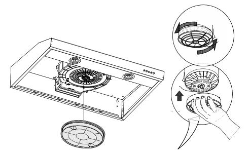
3. Install the grease filter. If replacement, please turn it in clockwise direction.
