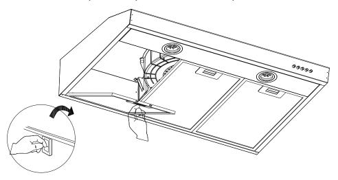
2. Push the LED lamp holder out from the cabinet by hand, or use screwdriver to prize up the LED lamp around the edges, pull out slotted the LED lamp and the wire together.
