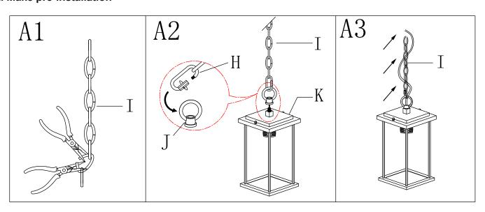
Step A1 » By measuring, determine the correct number of links needed for proper hanging height. Using the chain pliers, disconnect and discard the unwanted part.
