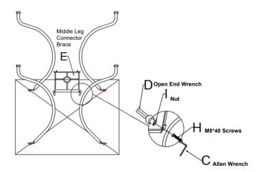
**STEP 2B:** Using the Open End Wrench (Part D) to hold the nut and the Allen Wrench (Part C) to turn the screws, securely tighten legs to the Middle Leg Connector Brace.
