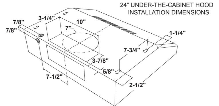
Exhaust outlet connects to 3-1/4" x 10" rectangular duct. Vent top or rear. Includes rectangular damper.
