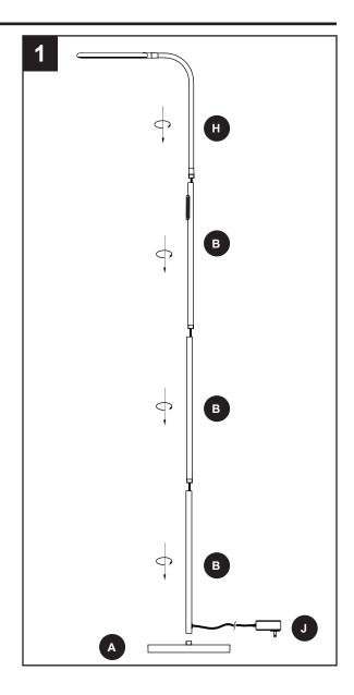
2. Plug the power adapter (J) into a grounded 120 V outlet.
